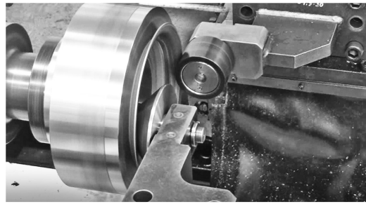
Fig. 6 Stator housing structure and example of flange processing with flow forming
