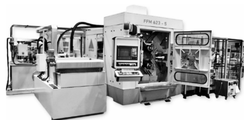
Fig. 4 The FFM machines use the backward flow-forming process to form weight-optimised rim rings. The cycle time is approximately 12 seconds.
